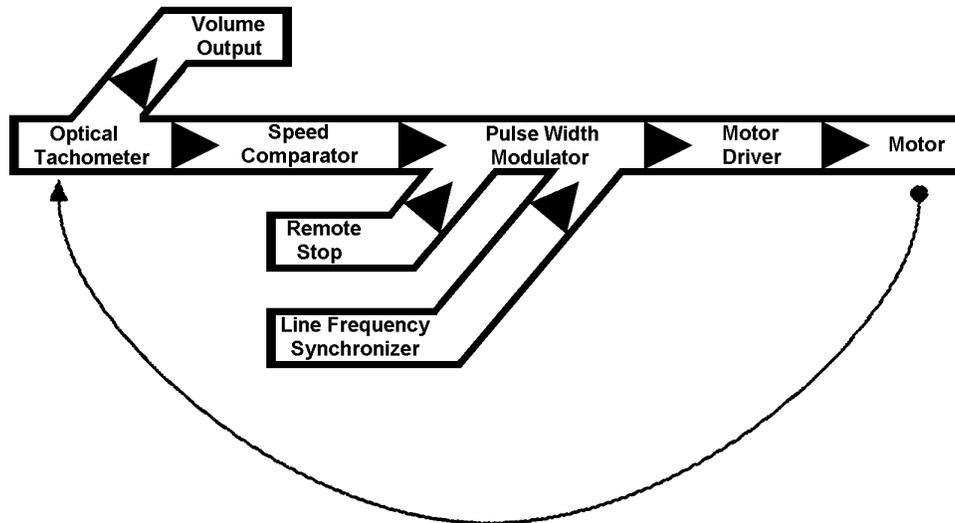
**Figure 5-2. MP-1 Electrical Block Diagram**
