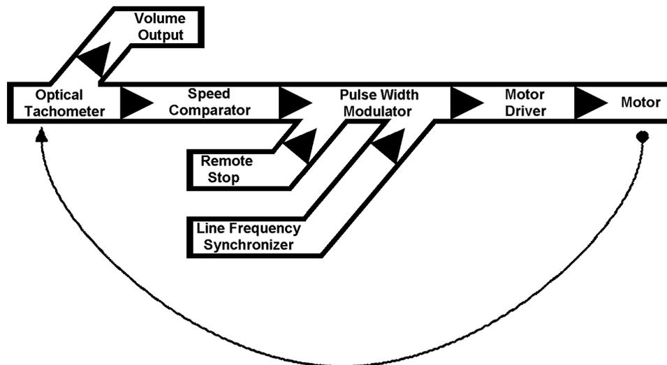
**Figure 7-2. MP-2 Electrical Block Diagram**
