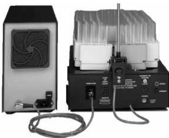
**Figure 3-7. Volumetric Collection Cable Connection**
