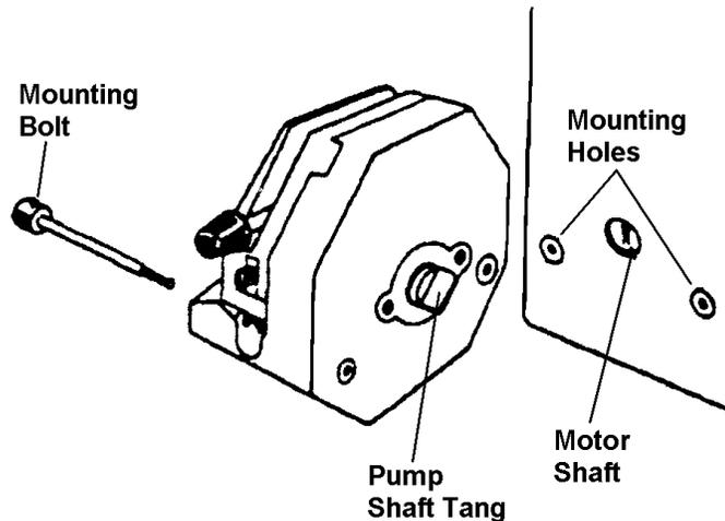
**Figure 2-1. Mounting a Single Fast-Load Pump Head**
