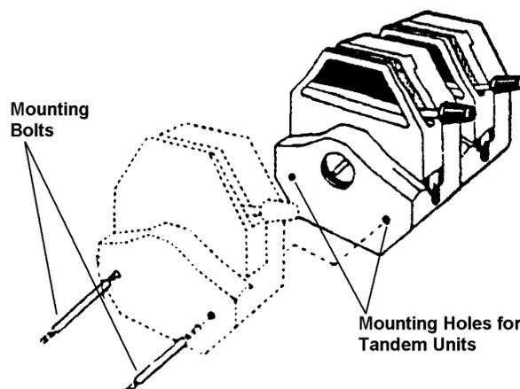
**Figure 2-2. Mounting Additional Fast-Load Pump Heads**
