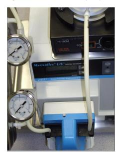
6. Connection is made by gently pushing the tubing onto the barbed fitting and turning the tubing cap clockwise until the tubing is secure.
