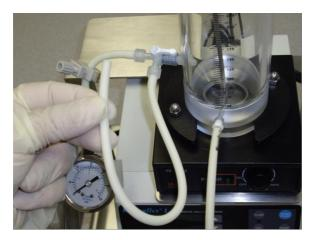
7. Place the other end of the tubing into a collection vessel.
