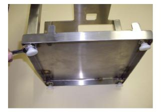
6. The TangenX<sup>™</sup> PRO PD LHV frame assembly is complete.
